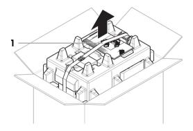
2 Open the lifting strap (1) and remove the User Manual (2).
